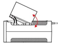
Aligned all arrows marks and slide the battery compartment cover back onto the battery housing. Double check if battery compartment is well-locked.
